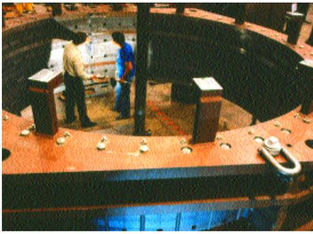
Laminated steel frames provide exceptional electrical response characteristics.
