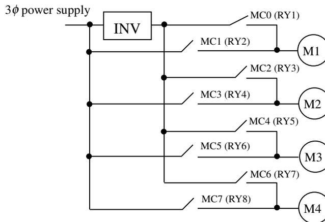
Fig 2 variable frequency pump cyclic mode.
