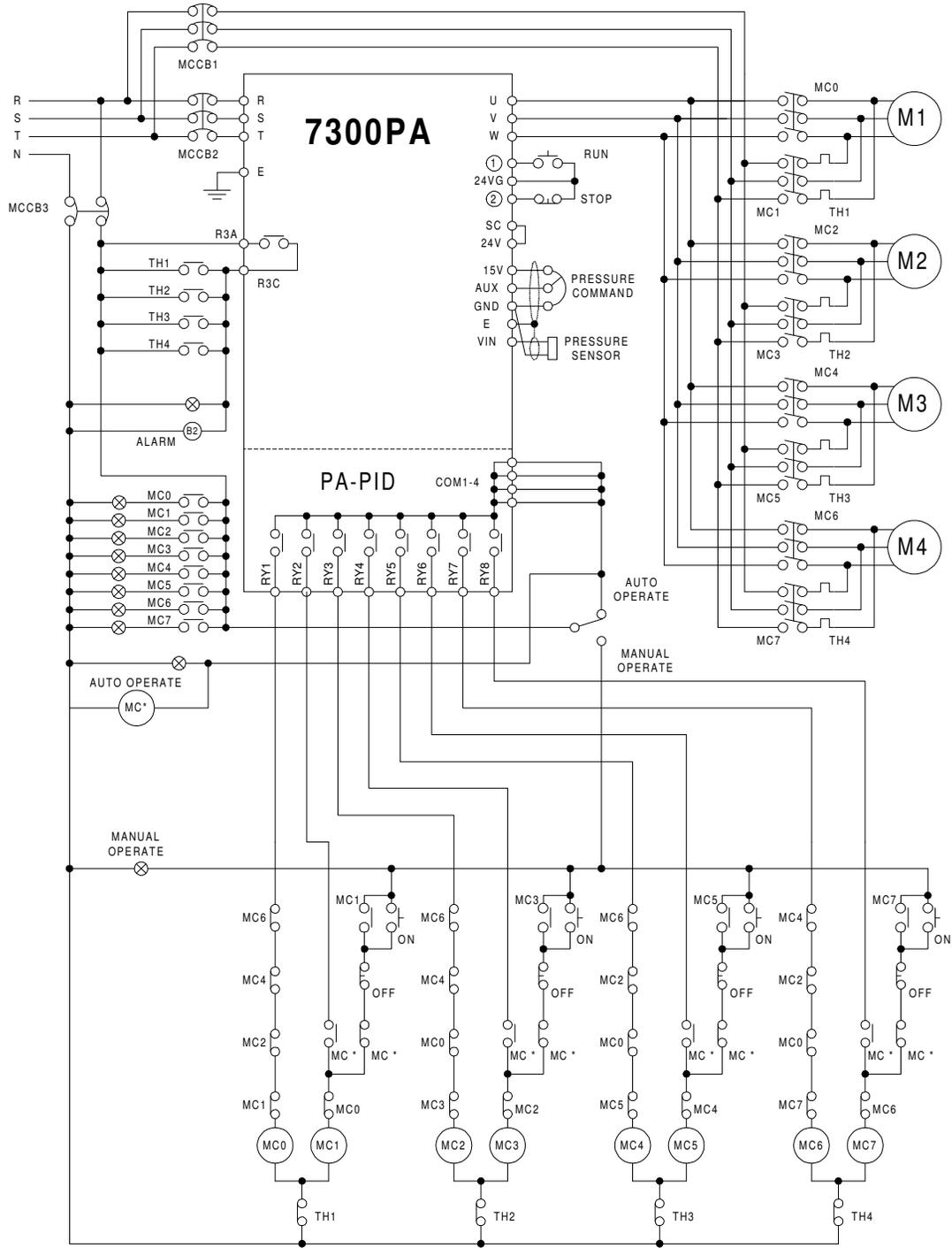
Fig 6 Fixed mode wiring diagram
